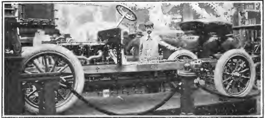
CHASSIS OF 50-HORSEPOWER PEUGEOT CAR AT PARIS SHOW.—NOTE REMOVABLE PAN BENEATH THE MOTOR AND TRANSMISSION.
